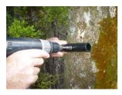
Using a 60mm roof screw in place of nail, attach pipe to tree leaving a small gap behind for the cover. The screw enables easy future adjustment for tree growth.
