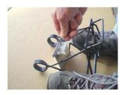
Holding trigger arm firmly, release grip from lifting bar and engage trigger arm hook with hole in trigger plate using free hand (not shown).
