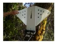
With trap attached and secured place cover behind pipe, adjusting gap if necessary using the screw.
