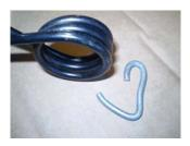
Safety catch can be portable or permanently crimped to trap.
