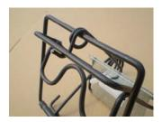
Incorrect location of trigger arm, TRAP CANNOT BE TRIPPED by possum.
