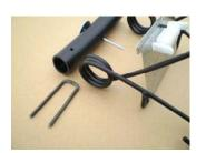
Drill hole through alkathene pipe to allow fitting of securing pin (best done with trap in place on the tree).
