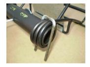
Correct location of securing pin preventing trap displacement upon capture
